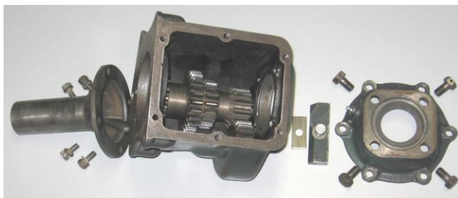
The open case - throwout bearing support tunnel, gear box, rear oil seal, U-joint housing
