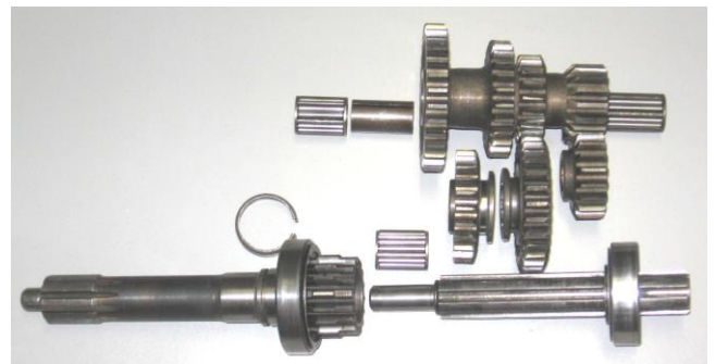
Transmission gears - cluster gear with bearings and spacer, 2nd, 1st, REV gears, input shaft, alignment bearing, gear slider and output shaft
